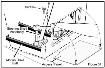
Remove the motion drive belt. A correct replacement part or assistance is available from an Authorized Service Center in your area.
